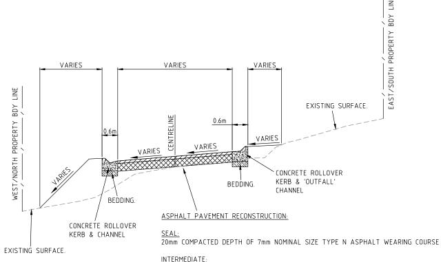
30mm COMPACTED DEPTH OF 10mm NOMINAL SIZE TYPE N ASPHALT BASE COURSE
