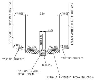
50mm COMPACTED DEPTH OF 10mm NOMINAL SIZE TYPE N ASPHALT WEARING COURSE
