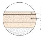
20mm COMPACTED DEPTH OF SIZE 7mm TYPE N ASPHALT WEARING COURSE 30mm COMPACTED DEPTH OF SIZE 10mm TYPE N ASPHALT WEARING COURSE 140mm COMPACTED DEPTH OF SIZE 20mm CLASS 2 CRUSHED ROCK 100mm COMPACTED DEPTH OF SIZE 20mm 3% CEMENT TREATED CLASS 3 CRUSHED ROCK EXISTING SIRGEADE
