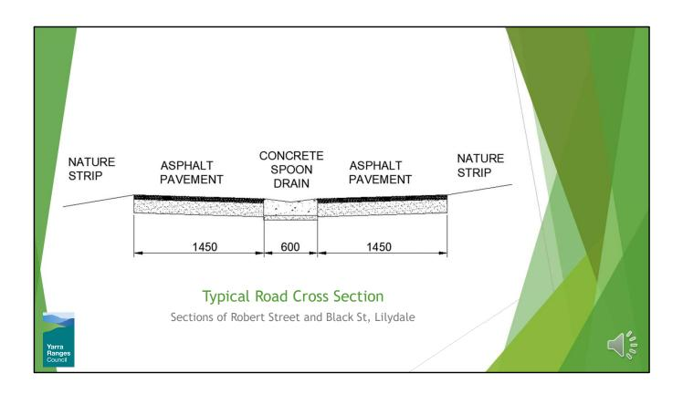
Here is a picture **Robert Street and Black Street's** cross sections with asphalt pavement and a centrally located concrete spoon drain.
