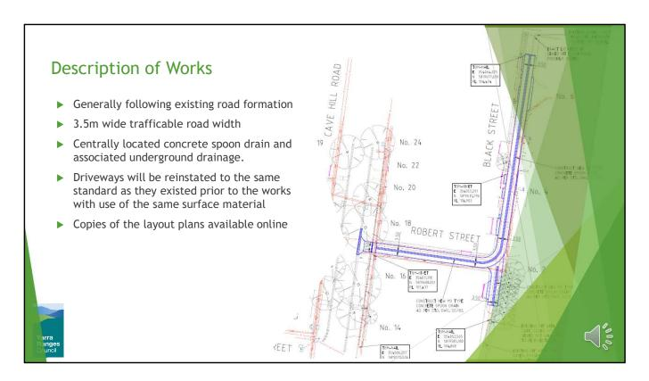
The description of works for Robert St and Black St, Lilydale, will be an Urban Standard 3.5m wide asphalt road with centrally located concrete spoon drain and associated underground drainage.
