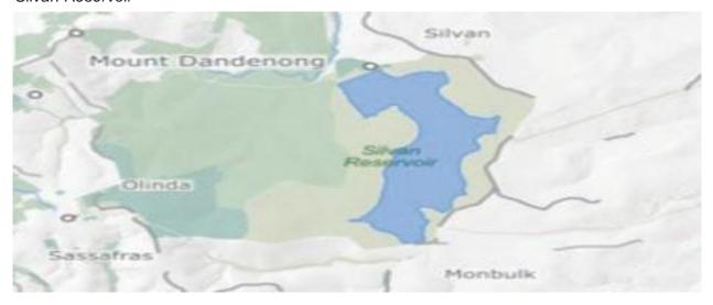
Silvan Reservoir is located in Silvan (approximately 40 kilometres east of Melbourne). Silvan is considered an off-stream storage reservoir as the main supply of water is provided by other catchments and reservoirs. The reservoir has a storage capacity of 40,000 megalitres and provides potable water supplies direct to townships as well as other storage reservoirs including Greenvale and Cardinia.
